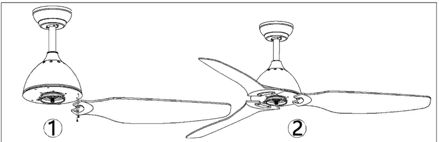
**6- Fitting the ceiling light.** Fit the metal light ring by fixing it in place under the blades
